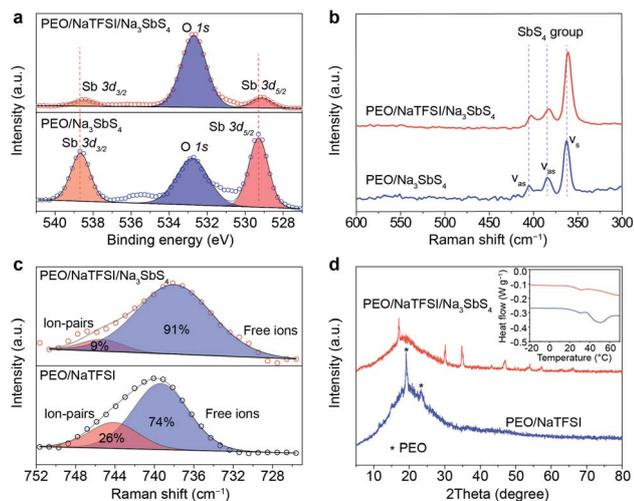
Fig. 3 Interactions between components in the PEO-based all-solid-state electrolytes. (a) Sb 3d XPS spectra and (b) Raman spectra of the PEO/ $Na_3SbS_4$  and PEO/NaTFSI/ $Na_3SbS_4$  electrolyte. (c) Raman spectra and (d) XRD patterns of the PEO/NaTFSI electrolyte and PEO/NaTFSI/ $Na_3SbS_4$  electrolyte. Inset: corresponding DSC curves.
