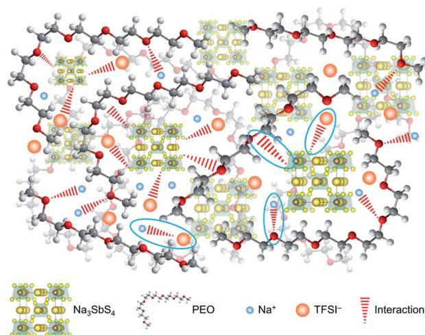
Fig. 4 Schematic diagram of the structure of the PEO/NaTFSI/ $Na_3SbS_4$  electrolyte, where the four types of interactions between the different components ( $Na_3SbS_4$  and TFSI<sup>-</sup>,  $Na_3SbS_4$  and PEO,  $Na^+$  and PEO,  $Na^+$  and TFSI<sup>-</sup>) are highlighted.
