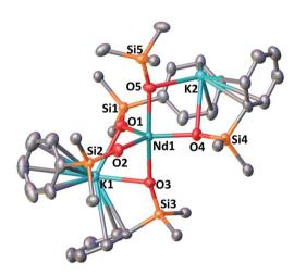
Fig. 2 Solid-state molecular structure of 2-Nd (50% probability ellipsoids). Hydrogen atoms, phenyl groups not bound to the potassium ions and residual solvent molecules are omitted for clarity. Selected distances (Å):  $Nd1-O_{siloxide}$  range = 2.206(2)-2.336(2); mean  $Nd1-O_{siloxide} = 2.28(4)$ ; Nd1-K1 = 3.6808(8); Nd1-K2 = 3.7774(8).
