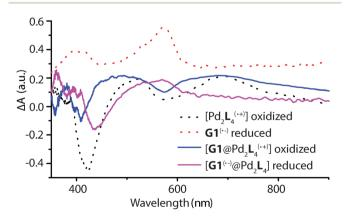
**Fig. 6** Electrochemically generated difference absorption spectra for the oxidized  $[Pd_2L^{(\cdot+)}_4]$ ,  $[G1@Pd_2L^{(\cdot+)}_4]$  and reduced  $G1^{(\cdot-)}$ ,  $[G1^{(\cdot-)}@Pd_2L_4]$  species (number of oxidized L units and overall charges not specified in formulas). UV-Vis spectra of samples recorded during cyclic voltammetry with a scan rate of 0.1 V s<sup>-1</sup>, Pt gauze as working electrode and Ag/AgNO<sub>3</sub> as reference electrode.
