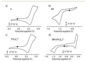
Fig. 5 Cyclic voltammograms of (a) ligand L (1.4 mM in DMSO), (b) guest G1 (0.35 mM in 0.1 M [NBu $_4$ ][PF $_6$ ] DMSO), (c) cage 1 (0.7 mM in 0.1 M [NBu<sub>4</sub>][PF<sub>6</sub>] DMSO) and (d) host-guest complex [G1@1] $^{2+}$ , (0.7 mM in 0.1 M [NBu<sub>4</sub>][PF<sub>6</sub>] DMSO), recorded at a glassy carbon working electrode against a  $Ag/AgNO_3$  reference electrode at 298 K. Scan rate 100 mV s<sup>-1</sup>.
