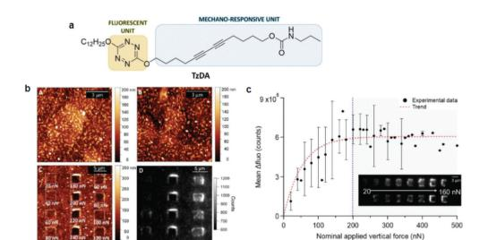
Fig. 5 (a) Schematic diagram of a molecular design of TzDA. (b) AFM morphology images of the (A) monomer, (B) polymer, and (C) polymer after mechanical stimulation. (D) Fluorescence image of poly-TzDA after the application of various forces. (c) A plot showing the recovered fluorescence signal vs. the applied vertical force. This figure has been adapted from ref. 48 with permission from the Royal Society of Chemistry, copyright 2019.
