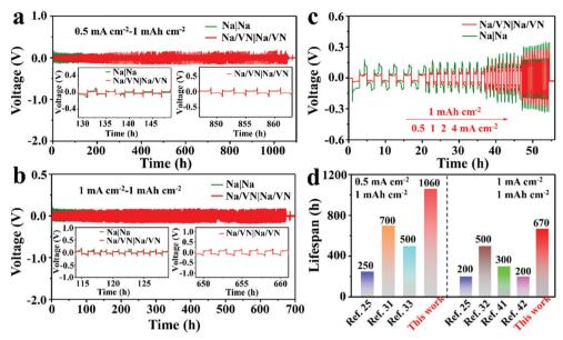
Fig. 2 Galvanostatic cycling of bare Na and Na/VN electrodes in symmetric cells (a) at 0.5 mA cm<sup>-2</sup> with 1 mA h cm<sup>-2</sup> and (b) at 1 mA cm<sup>-2</sup> with  $1 \text{ mA h cm}^{-2}$ . (c) Rate performance of Na/VN and bare Na symmetric cells at various current densities of  $0.5-4 \text{ mA cm}^{-2}$ . (d) A comparison of the lifespan of Na/VN with the previously reported Na metal anodes.
