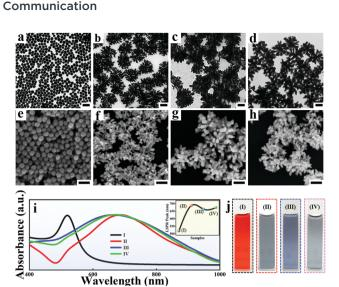
Fig. 2 TEM and SEM images of Au NPs (a and e), spiky AuNPs (b and f), spiky Au@Ag NPs (c and g) and etched-spiky Au@Ag NPs (d and g). (i and j) UV-vis spectra and optical photographs of the aqueous solution of Au NPs (I), spiky AuNPs (II), spiky Au@Ag NPs (III) and etched-spiky Au@Ag NPs (IV) (inset: LSPR peak location of the proposed four different NPs). The scale bar is 50 nm.
