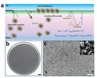
Fig. 3 (a) Schematic illustration of spiky Au@Ag NP monolayer films acquired at the oil-water interface. Optical photograph (b), SEM (c) and TEM (d) images of spiky Au@Ag NPs monolayer film. The scale bar is 1 cm (b), 20 µm (c) and 100 nm (d), respectively.
