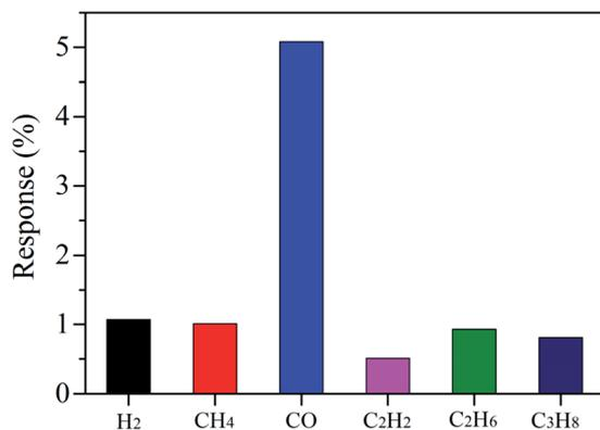
Fig. 11 Selectivity of the Ag-ZnO-MoS<sub>2</sub> nanocomposite sensor towards 100 ppm gas species of H<sub>2</sub>, CH<sub>4</sub>, CO, C<sub>2</sub>H<sub>2</sub>, C<sub>2</sub>H<sub>6</sub> and C<sub>3</sub>H<sub>8</sub> (reproduced from ref. 143 with permission from Elsevier).
