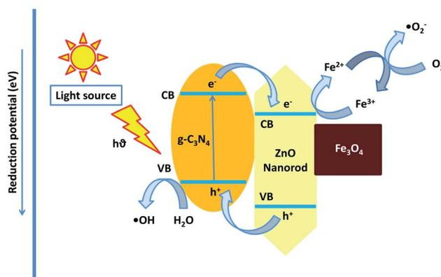
Fig. 27 Schematic depiction of the photocatalytic degradation mechanism of the g-C<sub>3</sub>N<sub>4</sub>/ZnO/Fe<sub>3</sub>O<sub>4</sub> heterojunction (reproduced from ref. 292 with permission from Elsevier).
