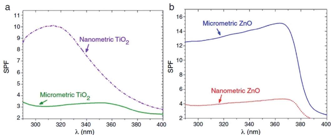
Fig. 16 SPF curves of COLIPA sunscreen incorporating an inorganic UV filter: nanometric (dashed lines) and micrometric (solid lines) (a)  $\text{TiO}_2$  and (b)  $\text{ZnO}$  particles (reproduced from ref. 149 with permission from Elsevier).
