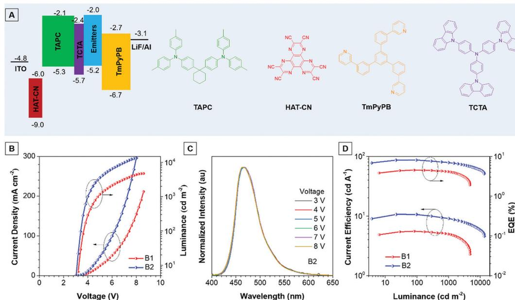
Fig. 4 (A) Device structure and ionization potentials (IPCV) and electron affinities (EACV) for each material. (B) Current density–voltage–luminance ( $J$ – $V$ – $L$ ) characteristics of devices B1 and B2. (C) Electroluminescence (EL) spectra of device B2 at various voltages. (D) CE and EQE versus luminance curves of the non-doped OLEDs based on the AIEgens TPA-An-Ph and TPA-An-mPhCz.
