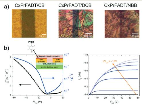
Fig. 7 a) From left to right, top view image of the OFETs based on cXPr-FADT films obtained by casting from a solution of chlorobenzene (CB), 1,2 dichlorobenzene (DCB) and n-butylbenzene (NBB), respectively. b) Transfer (left) and transport (right) plots measured to characterise the OFETs, with the device structure in the inset.
