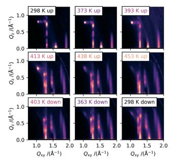
Fig. 2 2D scattering images obtained by GIWAXS measurements at different temperatures of evaporated C10-DNTT thin films. A clear change in the diffraction pattern can be observed above 400 K, which persists to over 453 K and during cooling down to room temperature.
