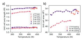
Fig. 5 a) Lattice constants a and b during heating  $(\triangleright, \triangle)$  and cooling  $(\triangleleft, \triangledown)$ . The filled triangles denote the high temperature polymorph II. It can be seen that the change in length is stronger for the b-axis in both polymorphs upon heating and cooling. b) The in-plane unit cell areas of both polymorphs plotted against the temperature. The filled in triangles denote polymorph II.
