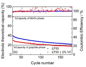
Fig. 9 Specific capacity and coulombic efficiency of #3 in LP30 (blue) and LP30 + 2% VC (red) and that of #2 in LP30 (green). (a) Rate capability test at different specific currents, and (b) stability test at 371 and 186 mA g<sup>-1</sup> in LP30 and LP30 + 2% VC, respectively
