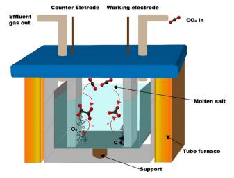
Fig. 1 Schematic of the MSCC-ET reactor.
