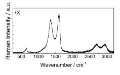
Fig. 4 (a) X-ray diffraction patterns of pristine synthesized carbon (red), C-50 (black) and diffractogram of Mn<sub>7.84</sub>O<sub>16</sub> (reference code 96-151-4117). (b) Raman spectrum of the carbon ground in an agate mortar.
