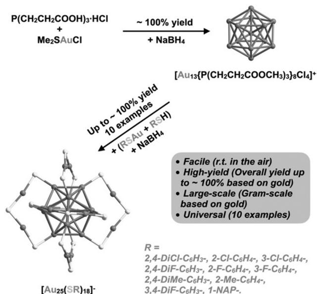
Fig. 16 Schematic illustration of cluster from cluster approach for the synthesis of AuNCs. Reproduced with permission.<sup>187</sup> Copyright 2021. Wiley-VCH.
