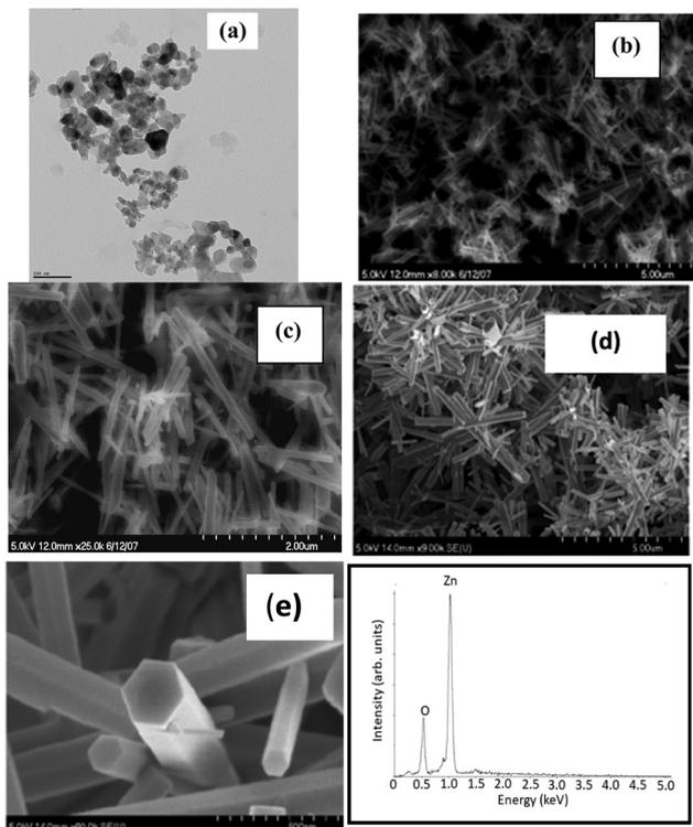
**Fig. 3** (a) TEM image of ZnO nanoparticles used as a seed layer for ZnO nanorods growth on a Si substrate with scale bar of 200 nm. (b) and (c) SEM images of ZnO nanorods grown in the solution phase without a seed layer, (d) and (e) ZnO nanorods grown on the pre-coated Si substrate with ZnO nanoparticles. (f) EDS spectrum of a ZnO nanorod sample grown on a Si substrate with the ZnO seed layer.
