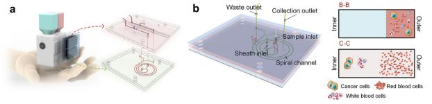
Fig. 7 (a) Conceptual design of the integrated chip for portable cancer cell separation. (b) Microfluidic chip presenting the spiral channel, sheath and sample inlets, collection and waste outlets. In the cross-sectional views of B-B and C-C, the cell migration along the channel respectively near the inlets and outlets is illustrated. Reproduced/adapted from ref. 175 with permission from the American Chemical Society.
