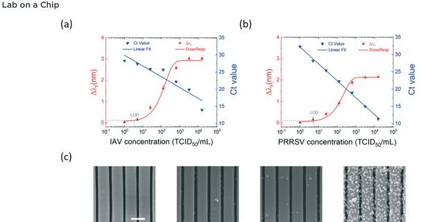
Fig. 5 Quantitative analysis of isolated IAV and PRRSV samples. (a) Measured  $\Delta \lambda_r$  as a function of isolated IAV concentration (red). The IAV titer was also measured using the RT-qPCR assay, and the Ct values were plotted (blue). (b) PC sensor response for the PRRSV titer (red) compared with the RT-qPCR Ct values (blue). (c) SEM images of the PC sensor surfaces after the adsorption of PRRSV-MNP at different PRRSV concentrations (scale bar: 555 nm).
