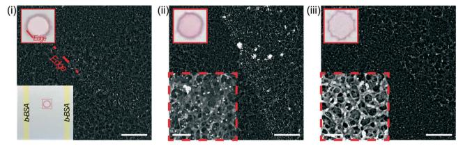
Fig. 6 SEM images obtained at the edge of the (i) as-printed spots and after a 5 minute incubation on the (ii) benchtop orbital shaker with shear rate  $\sim 10^{1}$  s<sup>-1</sup> or (iii) using fast CD LR with shear rate  $\sim 10^{3}$  s<sup>-1</sup> (scale bar: 10  $\mu$ m; inset scale bar: 2  $\mu$ m). Dashed inset at higher magnification and solid inset of regular image illustrating spot deformation cause by fast flow.
