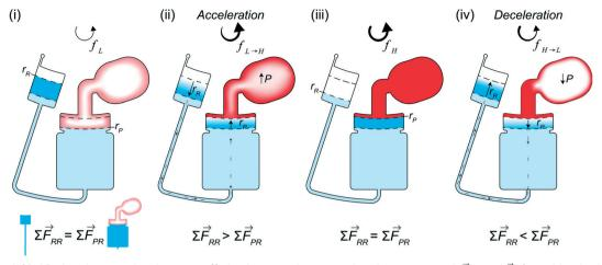
Fig. 2 Stages of CD LR. At a low rotation frequency (i) the forces acting on each column are equal  $(\vec{F}_{RR})$  resulting in the liquid radial positions  $r_R$  and  $r_P$ . Acceleration (ii) increases the centrifugal force, causing liquid to flow from the RR to the PR and the pressure in the GC to increase until the high rotation frequency (iii). Deceleration reverses the process (iv).
