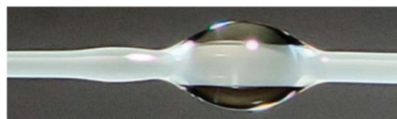
Fig. 5 Droplets of solvent on fiber spun from PAN in DMSO solution showing phase separation of the stretched polymer (in white) and the solvent (transparent droplet). Reproduced from ref. 76 with permission from Wiley-VCH Verlag GmbH & Co. KGaA.
