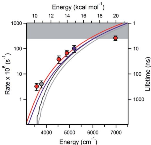
Fig. 4 The measured (points) and various theoretically predicted  $k(E)$  (curves) for QOOH  $\rightarrow$  OH + oxetane. The highest energy point is hitting the experimental time-resolution (gray band). Reproduced from *Faraday Discussions* (<https://doi.org/10.1039/d2fd00008c>) with permission from the Royal Society of Chemistry.
