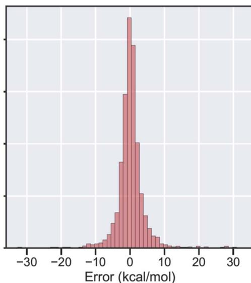
Fig. 8 Histogram of the errors in our fast estimator of zpe-corrected reaction barrier height  $\Delta E_0$  relative to high-accuracy CCSD(T)-F12a/cc-pVDZ-F12//wB97X-D3/def2-TZVP values for about 2000 reactions not included in the training set. The mean absolute error in the estimates is  $<3$  kcal mol $^{-1}$ , smaller than the average error in DFT calculations of these barriers.
