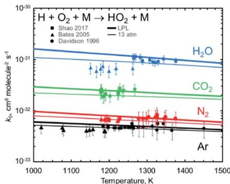
Fig. 1 Predicted vs. experimental rate coefficients for  $\text{H} + \text{O}_2 + \text{M} \rightarrow \text{HO}_2 + \text{M}$  near the low-pressure limit, showing how well Jasper's *ab initio* method works for predicting the dependence on bath gas composition (the identity of M). Reproduced from *Faraday Discussions* (<https://doi.org/10.1039/d2fd00038e>) with permission from the Royal Society of Chemistry.
