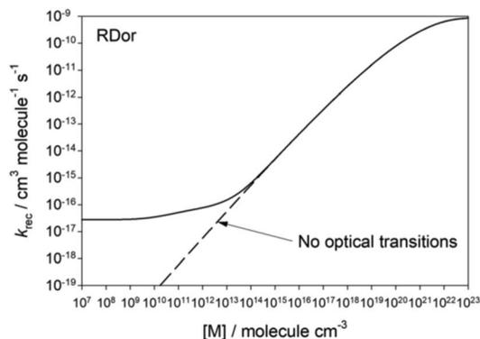
Fig. 12 Predicted variation in the rate coefficient for  $\text{SiO}_2 + \text{H}_2\text{O} \rightarrow \text{OSi}(\text{OH})_2$  as a function of pressure, at conditions relevant to the region near the star RDor. At low pressures the excited adduct is cooled primarily by radiation. Reproduced from *Faraday Discussions* (<https://doi.org/10.1039/d2fd00025c>) with permission from the Royal Society of Chemistry.
