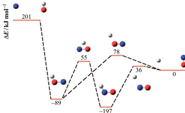
Fig. 1 Energy diagram for reaction (1) and its intermediates (blue, red, and white spheres symbolize N, O, and H atoms, respectively; the energies  $\Delta E$  relative to H + NO are adapted from ref. 19 and 41).
