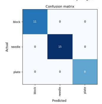
Fig. 7 Confusion matrix of morphology labels assigned by the labelling robot using a deep learning model trained on the "in house" experimental dataset.
