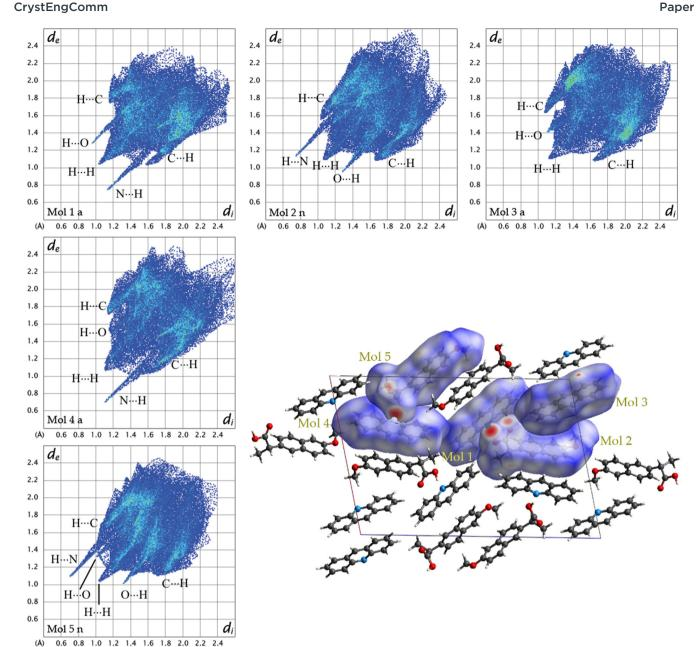
Fig. 6 Fingerprint plots for each symmetry-independent molecule in  $1\alpha$  and crystal structure model of 1a viewed along the b-axis showing Hirshfeld surfaces with d-norm plotted.
