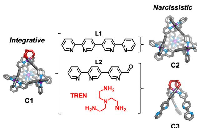
**Scheme 1** Left: Self-assembly of a heteroleptic tetrahedral cage **C1** by integrative sorting. Right: Formation of homoleptic cage **C2** and the mononuclear complex **C3**. Exclusive formation of **C1** or social sorting is possible when using **L1**, **L2**, TREN and Fe(II) starting materials.
