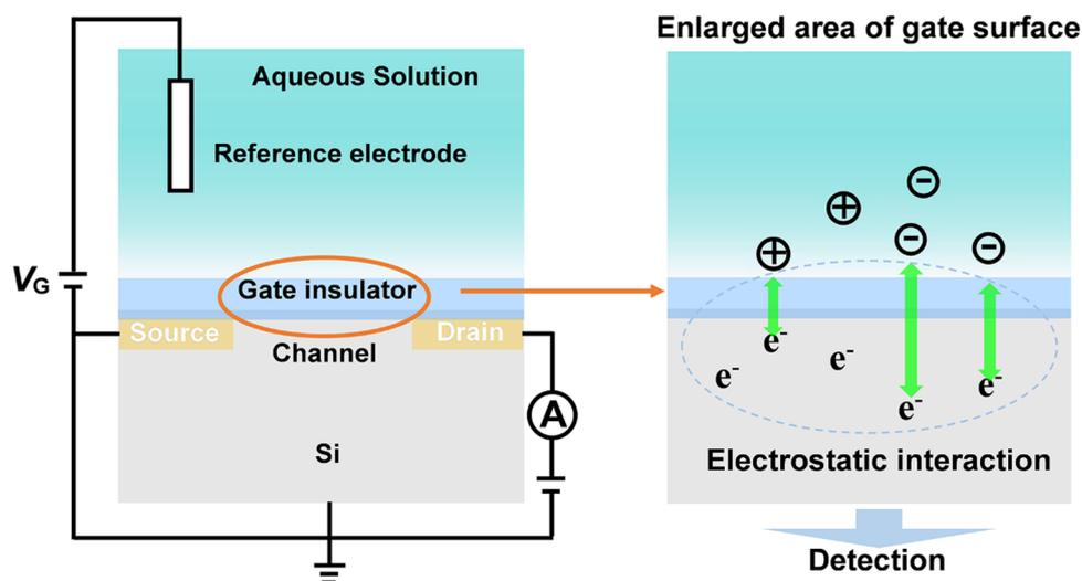
Fig. 10 Structure and principles of Bio-FETs.
