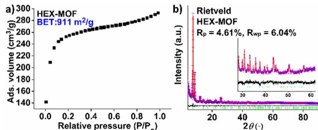
Fig. 1 (a)  $N_2$  sorption isotherm (77 K) for **HEX-MOF**. (b) Rietveld plot of **HEX-MOF**. Violet crosses: experimental points; red line: calculated pattern; black line: difference pattern (exp-calc); and green bars: Bragg positions. Inset: Magnification of the  $2\theta$  region 30–60°.
