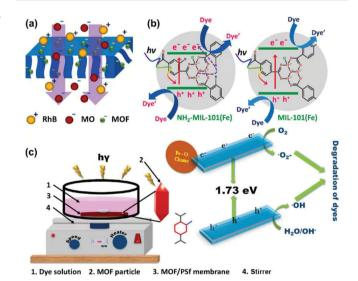
Fig. 10 Schematic illustration of (a) rejection and (b) photocatalytic degradation of dye molecules over the NH2-MIL-101(Fe) and MIL-101(Fe) MOF-integrated membranes and (c) pictorial illustration of degradation setup and its mechanism. Reproduced from ref. 139 with permission from Elsevier Inc, copyright 2022.
