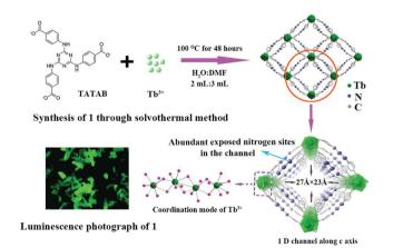
Fig. 4 Schematic for the formation of Tb-MOF for the adsorption and detection of uranium from aqueous solution. Reproduced from ref. 106 with permission from American Chemical Society, copyright 2017.
