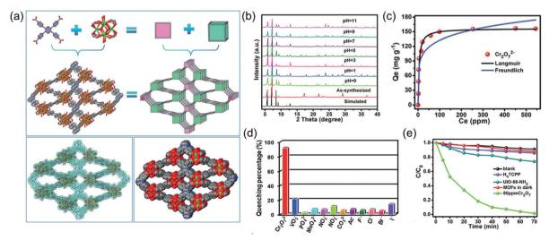
Fig. 6 (a) The structure illustration of JLU-MOF60; (b) the stability of JLU-MOF60 in various pHs; (c) the removal ability; (d) the sensing ability and (e) the degradation ability of JLU-MOF60 for  $Cr_2O_7^{2-}$  treatment. Reproduced from ref. 122 with permission from Royal Society of Chemistry, copyright 2019.
