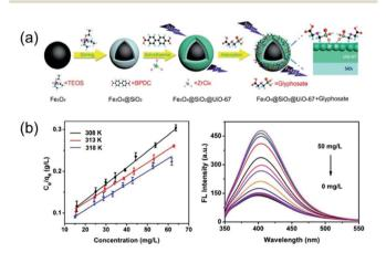
Fig. 11 (a) A schematic illustration of the fabrication of the  $Fe_3O_4$ @-SiO\_2@UiO-67 MOF-based adsorbent. (b) The adsorption and the detection performance for glyphosate treatment. Reproduced from ref. 147 with permission from Royal Society of Chemistry, copyright 2018.
