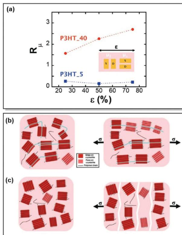
Fig. 11 (a) Anisotropy in the field-effect mobility ( $R_H$ ) of transistors utilizing **P3HT\_40** and **P3HT\_5** thin films, as a function of strain. Schemes of unstrained and strained (b) **P3HT\_40** and (c) **P3HT\_5**, highlighting the role of tie chains between the crystallites on polymer morphology upon strain. Reproduced with permission from Wiley.<sup>91</sup>
