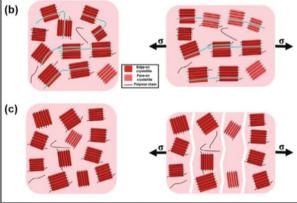
Fig. 11 (a) Anisotropy in the field-effect mobility  $(R_{\mu})$  of transistors utilizing P3HT\_40 and P3HT\_5 thin films, as a function of strain. Schemes of unstrained and strained (b) P3HT\_40 and (c) P3HT\_5, highlighting the role of tie chains between the crystallites on polymer morphology upon strain. Reproduced with permission from Wiley.91
