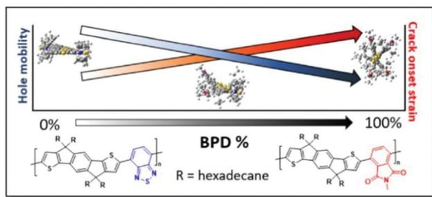
Fig. 10 Chemical structures of **PIDTBTBTD** and **PIDTBPB** in the copolymers with various percentages of BPD unit (along with the respective DFT geometries), and the trends of hole mobility and CoS dependence on the BPD share. Reproduced with permission from American Chemical Society.<sup>38</sup>
