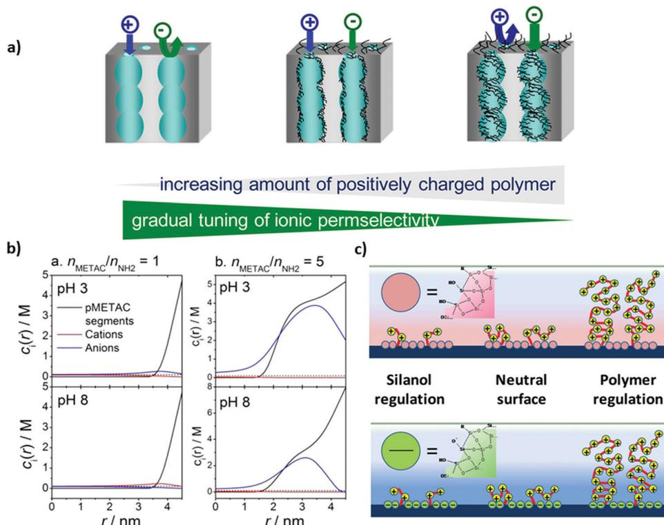
Fig. 4 (a) Schematic depiction of mesoporous silica thin films functionalized with PMETAC at various electrolyte density, (b) molar concentration of polymer segments, cations ( $\text{K}^+$ ) and anions ( $\text{Cl}^-$ ), as a function of the distance from the center of the pore, and (c) schematic depiction of the modified silica surface at acidic pH  $< 3$  (upper figure) and alkaline pH  $> 7$  (lower figure). Reprinted with permission from ref. 134 Copyright (2015), American Chemical Society.
