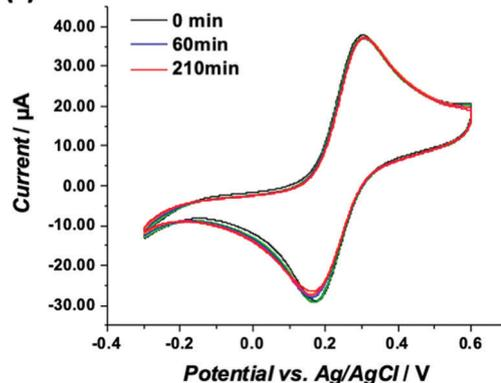
Fig. 4 CVs measured for the (a) NMPA SAM, (b) 1-hexanethiol SAM and (c) bare Au in 1 mM  $K_4[Fe(CN)_6]$ . Experimental conditions: 10 mM PBS buffer pH 7 containing KCl 2.7 mM and NaCl 137 mM; scan rate  $100 \text{ mV s}^{-1}$  and  $T = 25 \text{ }^\circ\text{C}$ . Each panel reports curves acquired on the same sample monitoring the cyclic voltammograms for a total time of 210 min. The red arrows point in the direction of the peak shift.
