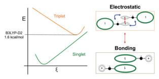
Fig. 10 Left: Scheme of the potential energy landscape of the singlet and triplet states along the reaction coordinate that drives the spin transition. The adiabatic energy gap computed at B3LYP-D2 level is indicated. Right: Scheme of the electronic configuration and intermolecular interactions dominating the stability of the LS (bonding) and HS (electrostatic) states.
