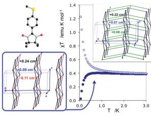
Fig. 4 Calculated magnetic susceptibility  $\chi T(T)$  data for p-(methylthio)-phenyl nitronyl nitroxide (see chemical formula inset, where hydrogen atoms are omitted for clarity) using the magnetic topology at 298 K (2D layer with competing FM and AFM interactions) and at 10 K (purely bulk FM).
