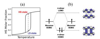
Fig. 1 (a) Schematic representation of the evolution of the high spin (HS) molar fraction upon increasing temperature. Inside the hysteresis region, both the low spin (LS) and HS states can be obtained (i.e. bistability). (b) Diagram of the frontier molecular orbitals of a pancake bond. The  $\pi$ -dimer of tetrathiafulvalene radical cation is shown where HOMO and LUMO orbitals are depicted.
