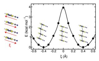
**Fig. 16** Potential energy profile of an isolated stack of 4-NCBDTA radicals along the reaction coordinate,  $\xi$ , defined in the left-most scheme.  $\xi$  describes a collective sliding motion of the radicals that preserves the inter-planar distance between them. The profile was computed with periodic boundary conditions along the stacking direction. The regular structure shown at  $\xi=0$  corresponds to the regular stack of the crystal structure at 300 K.
