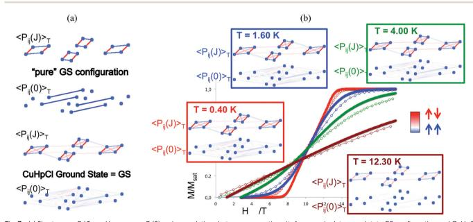
Fig. 7 (a) Short-range  $P_{ii}(J)_T$  and long-range  $P_{ii}(0)_T$  spin correlations between magnetic units for pure singlet ground state GS configuration and CuHpCl ground state GS configuration. (b) Temperature dependence of the magnetic correlation between all spin units at 0.40, 1.60, 4.00, and 12.30 K (in accordance to the magnetization experimental data). Notice that spins coupled are represented in red, and spins arranged parallel in blue.
