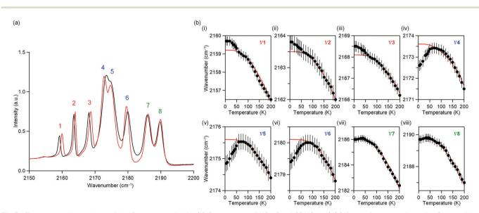
Fig. 3 Temperature dependence of the IR spectrum of MnW. (a) IR spectrum at 5 K (red) and 60 K (black). (b) IR peak frequency due to the CN stretching mode,  $\nu_i$  (i = 1-8), vs. temperature plots. Red line indicates the peak position obtained by fitting the theoretical equation of thermal expansion<sup>61</sup> due to anharmonic phonons without magnetic ordering. Error bars indicate the resolution of the apparatus.
