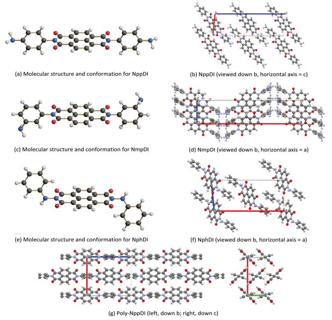
Fig. 2 Schematic drawings of the molecular structure and crystal packings of (a and b) NppDI, (c and d) NmpDI and (e and f) NphDI, together with a note of their orientations. In (g), the polymeric poly-NppDI structure is shown. Color codes: C in grey, N in blue, O in red and H in white. Graphics realized by Schakal<sup>42</sup> (a, c and e) and Mercury<sup>43</sup> (b, d, f and g).
