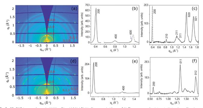
Fig. 9 2D-GIXD images of annealed (a) NmpDI and (d) NphDI thin films recorded for  $\alpha_i = 0.1^{\circ}$ . The corresponding integrated intensity profiles along  $q_{z_i}$ [(b and e)], and along  $q_{xy}$ , [(c and f)] are reported. The dashed lines in b, c and e are Gaussian fits to the experimental data at the positions where the detector cuts hamper collection of the diffracted intensity
