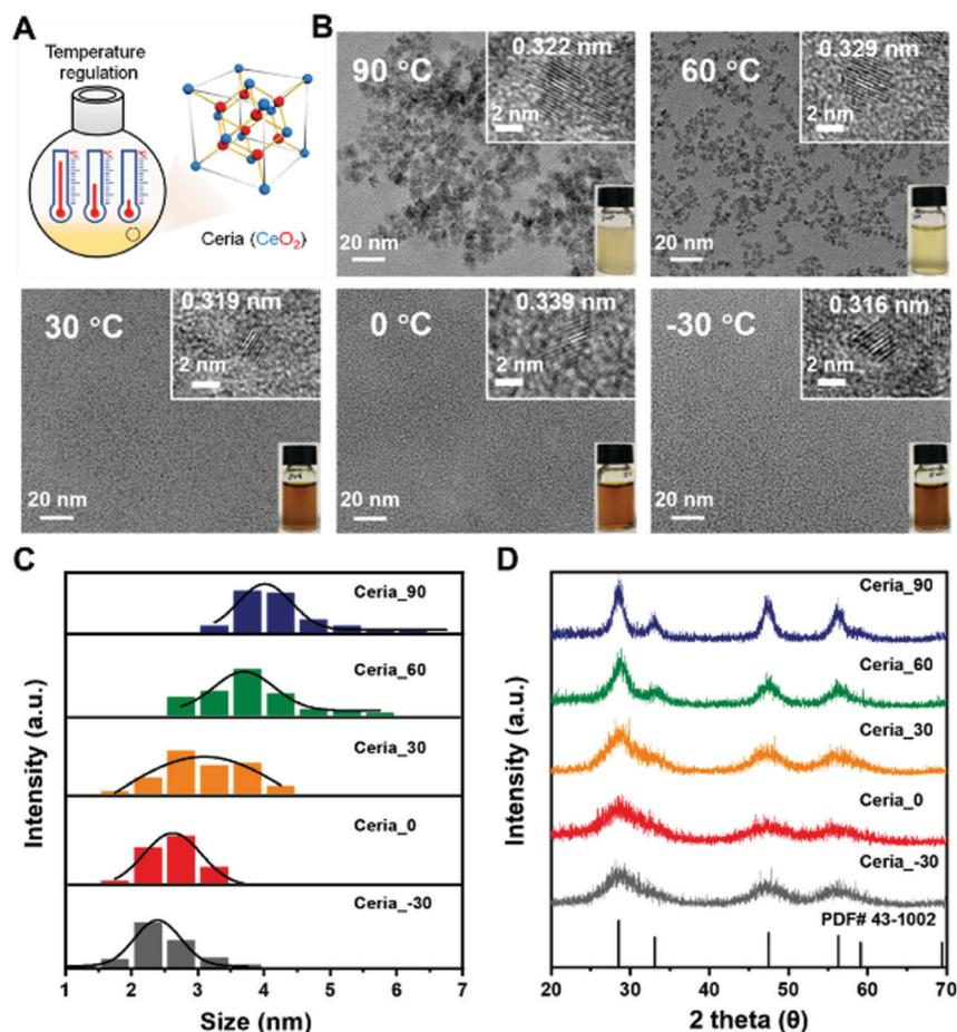
Fig. 2 Synthesis scheme (A) and characterization (B–D) of different CeO<sub>2</sub> samples: (B) TEM images, (C) size distribution histograms of CeO<sub>2</sub> measured from TEM images, and (D) XRD patterns.
