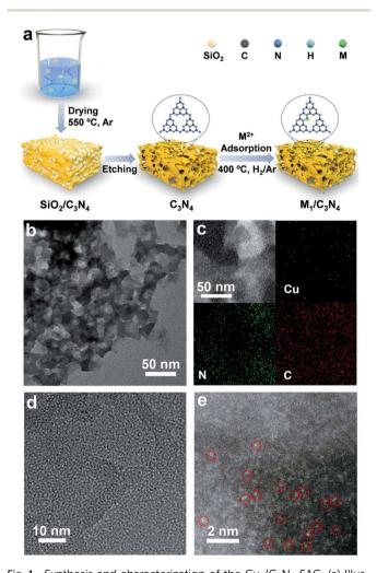
Fig. 1 Synthesis and characterization of the  $Cu_1/C_3N_4$  SAC. (a) Illustration of the synthetic route to  $M_1/C_3N_4$ . (b) TEM image of  $Cu_1/C_3N_4$ . (c) HAADF-STEM and corresponding elemental mapping images of  $Cu_1/C_3N_4$  showing the uniform distribution of Cu (yellow), N (green) and C (red). (d and e) High-resolution TEM image (d) and AC HAADF STEM image (e) of  $Cu_1/C_3N_4$  (single Cu atoms are marked with red circles).
