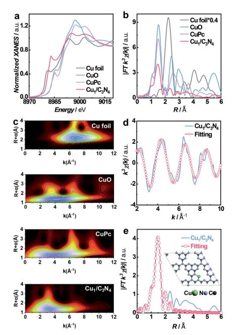
Fig. 2 XAS analysis of  $Cu_1/C_3N_4$ . (a and b) Normalized XANES spectra (a) and FT-EXAFS spectra (b) at the Cu K-edge of  $Cu_1/C_3N_4$  (red line), Cu foil (black line), CuO (blue line) and CuPc (purple line). (c) Wavelet transforms of the Cu K-edge EXAFS spectra for Cu foil, CuO, CuPc and  $Cu_1/C_3N_4$ . (d and e) Corresponding fitting curves of the EXAFS spectra of  $Cu_1/C_3N_4$  in k space (d) and R space (e). The inset in (e) is the schematic structure of  $Cu_1/C_3N_4$ .
