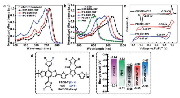
Fig. 2 UV-vis absorption spectra of the polymers and NFAs in (a) chlorobenzene solution and (b) film. (c) Cyclic voltammograms of NFAs, (d) chemical structures of PBDB-T and PM6, and (e) energy level diagram of polymers and NFAs.
