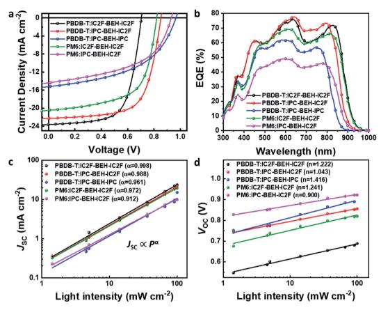
Fig. 5 (a) J-V curves and (b) EQE spectra of PBDB-T:NFA and PM6:NFA-based OSCs. (c) Plot of  $J_{SC}$  vs. light intensity and (d)  $V_{OC}$  vs. light intensity for the OSCs.
