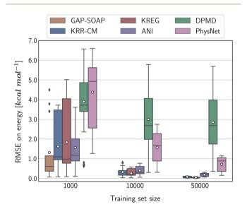
Fig. 4 Box plot representation of the MLPs' learning performance across the compositional space of the MD17 database. All ML models were trained only on energies. Each box plot represents the distribution of the root-mean-squared error (RMSE) for the total energies of all molecules in the MD17 database calculated with respect to the true labels of a test set with 20k geometries. The white dots in the box plots correspond to the mean value of the RMSE for all different molecules.
