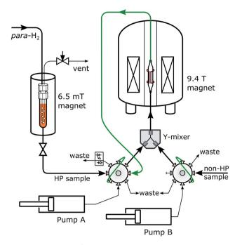
Fig. 2 Instrument for SABRE NMR measurements of ligand binding. The putative ligand interacts with *para*-hydrogen and polarization transfer catalyst at 6.5 mT. It is subsequently delivered to a sample loop. The ligand and protein samples are pushed by high-pressure syringe pumps through the Y-mixer, to a flow-cell in the NMR magnet, where the measurement takes place.
