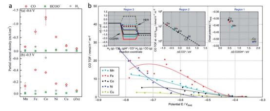
Fig. 1 (a) The volcano trend of M-N-C catalysts in terms of electrochemical CO<sub>2</sub>RR performance. Partial current densities of M-N-C catalysts for CO, HCOO $^-$ , and H<sub>2</sub> products at -0.6 V<sub>RHE</sub> and -0.5 V<sub>RHE</sub>. Reproduced from ref. 56 with permission from the American Chemical Society, copyright 2019. (b) Experimental CO TOFs of M-N-C catalysts. Reproduced from ref. 40 with permission from Springer Nature, copyright 2017.
