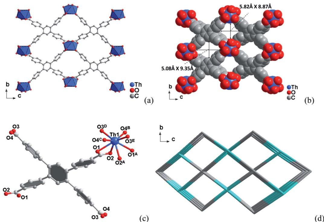
Fig. 1 (a) Three-dimensional framework structure of compound 1 along the  $a$  axis. (b) The corresponding space-filling models with the pore diameters obtained by taking the van der Waals radii. (c) Coordination environments of the Th(IV) sites in compound 1. (d) Topology framework for compound 1 showing the channels along [100] direction.
