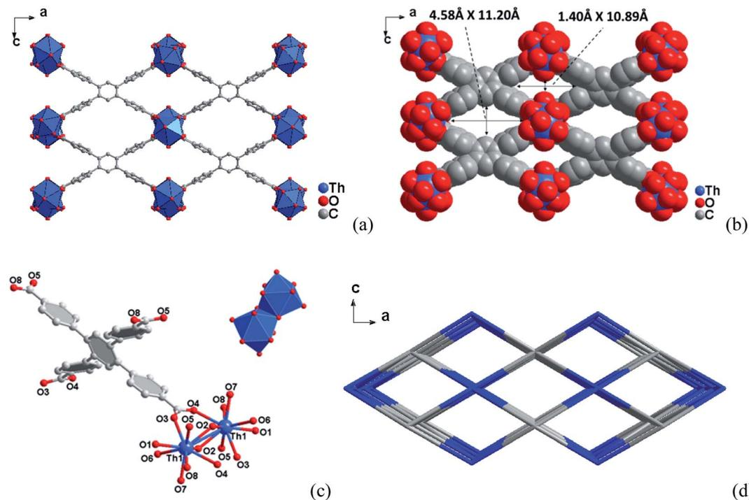
Fig. 2 (a) View along the *b* axis of the structure of compound 2. (b) The corresponding space-filling models with the pore diameters obtained by taking the van der Waals radii. (c) Coordination environments of the Th(IV) sites in compound 2 and dimer of Th<sub>2</sub>O<sub>3</sub>(H<sub>2</sub>O)<sub>4</sub>(CO<sub>2</sub>)<sub>2</sub>(CO)<sub>4</sub>. (d) Topology framework for compound 2 showing the channels along [010] direction.
