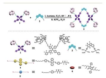
Scheme 1 Self-assembly of 120° dipyridyl donor 1 and 60° diplatinum (II) acceptor 2 into discrete rhomboidal metallacycle 3, and the chemical structures of building block DSA-containing guest 4, model guest 5 and fluorescent acceptor 6.
