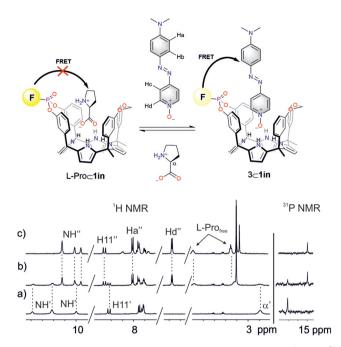
Fig. 8 (Top) Competitive IDA binding equilibrium. (Bottom) <sup>1</sup>H and <sup>31</sup>P NMR spectra of a 2 mM solution of L-Pro⊂1in in CD2Cl2 after the addition of 0 (a), 0.5 (b) and 1.0 (c) equiv. of 6. F denotes the fluorophore: phenyl-amino-naphthyl group.
