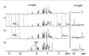
Fig. 4 <sup>1</sup>H NMR (400 MHz, 298 K) and <sup>31</sup>P NMR spectra of a 2 mM CD<sub>2</sub>Cl<sub>2</sub> solution of 1in before (a) and after (b-d) solid-liquid extraction with solid L-Pro (b) and solid L-Pip (c) and with equal amounts of solid L-Pro and L-Pip (d).
