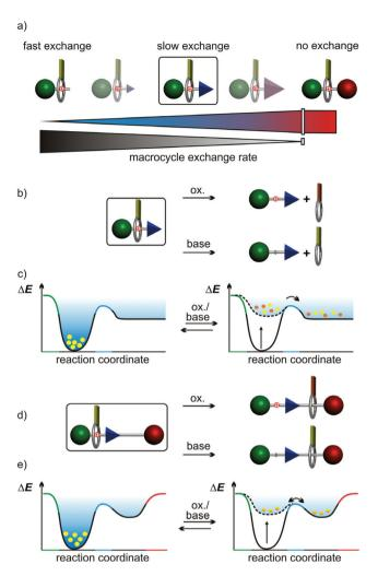
Fig. 1 (a) Range of macrocycle exchange rates from a quickly reversible pseudorotaxane formation (light blue, small 'speed bump') to a fully interlocked rotaxane (red stopper). (b) Stimuli-induced shuttling or unthreading and (c) the corresponding changes of the energy landscapes of a pseudorotaxane as well as (d and e) of a rotaxane (stoppers: green/red, steric 'speed bump' in the axle: blue, TTF oxidation states in yellow (reduced)/orange (oxidized to TTF<sup>2+</sup>).
