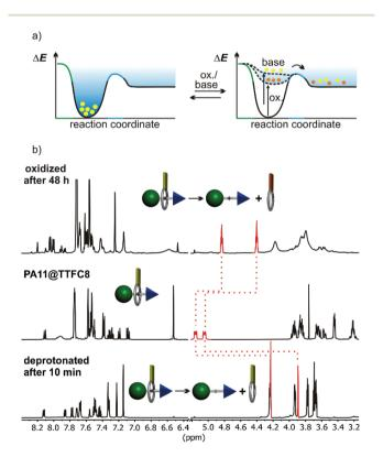
Fig. 5 (a) Dual-stimuli switching expressed in terms of the potential energy surface of the pseudorotaxane PA11@TTFC8. (b)  $^{1}$ H NMR spectra (600 MHz, dry CD $_{2}$ Cl $_{2}$ , 298 K) of PA11@TTFC8 (center), 48 hours after oxidation with excess NOSbF $_{6}$  (top), and 10 minutes after deprotonation with an excess of Schwesinger's P2 base immobilized on polystyrene (bottom).
