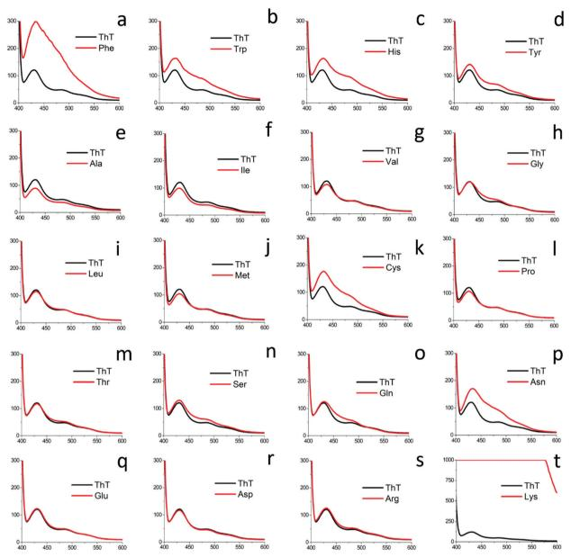
ThT fluorescence assay for all naturally occurring amino acids at 80 mM concentration using optimized ThT concentration.
