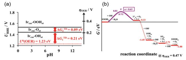
Fig. 5 Theoretical studies for OH<sup>-</sup> oxidation over iridium oxide. (a) The ab initio Pourbaix diagram for a single-crystalline IrO<sub>2</sub>(110). (b) The free energy diagram over IrO<sub>2</sub>(110) in alkaline media (pH = 12.9) at an OER overpotential of 0.47 V. Reprinted with permission from ref. 95. Copyright (2019) American Chemical Society.
