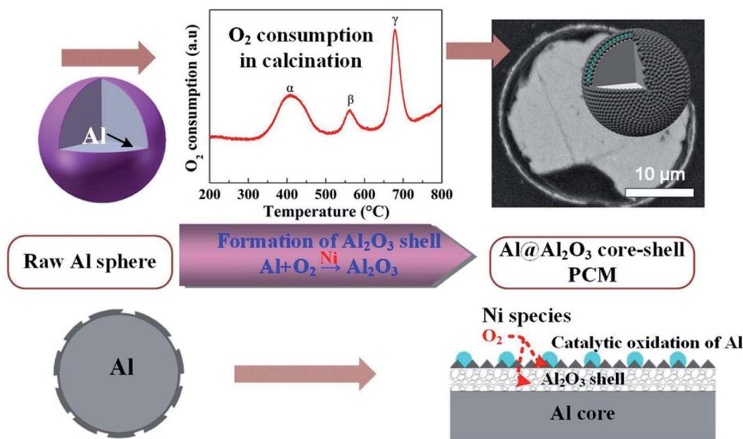
Fig. 15 Synthesis of Al@Al<sub>2</sub>O<sub>3</sub> microcapsule for high-temperature TES.<sup>103</sup> Reproduced from ref. 103 with permission of The American Chemical Society, Copyright 2018.
