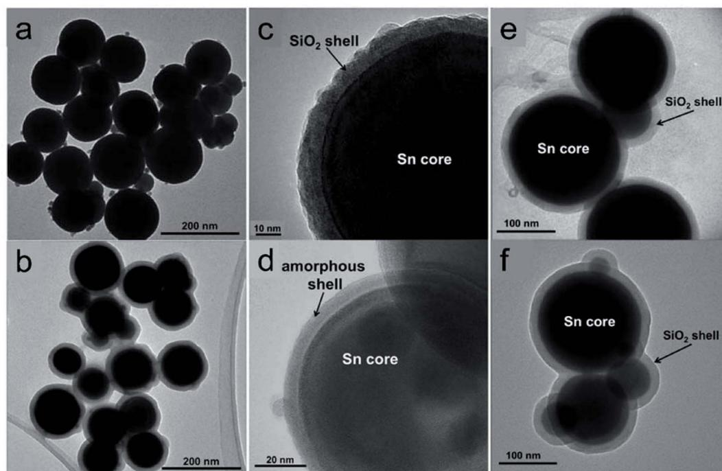
Fig. 6 Silica encapsulated Sn nanoparticles (Sn@SiO<sub>2</sub>) for heat transfer and TES.<sup>84</sup> TEM images of (a) as-prepared Sn and (b) Sn@SiO<sub>2</sub> nanoparticles; high-resolution TEM images of (c) Sn@SiO<sub>2</sub> and (d) Sn nanoparticles. TEM images of encapsulated Sn@SiO<sub>2</sub> nanoparticles (e) before and (f) after 20 heating and cooling cycles. Reproduced from ref. 84 with permission from Wiley, USA, Copyright 2013 John Wiley & Sons, Ltd.
