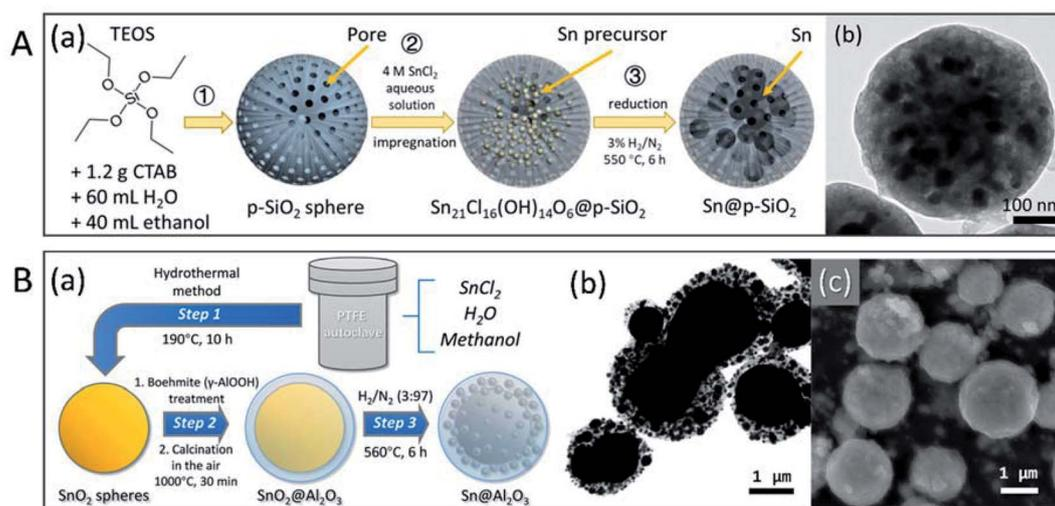
**Fig. 8** Micro and nano encapsulated Sn-based PCM particles. (A) Sn NPs@p-SiO<sub>2</sub>: (a) 3-step synthesis method, (b) TEM image; (B) size-tunable Sn@Al<sub>2</sub>O<sub>3</sub>: (a) 3-step synthesis method, (b) TEM and (c) SEM images of Sn@Al<sub>2</sub>O<sub>3</sub>. Reproduced from ref. 88 and 89 with permission of The American Chemical Society, Copyright 2018 and 2019, respectively.
