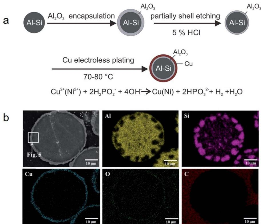
Fig. 16 (a) Synthesis method to obtain Al-25 wt% Si@Al<sub>2</sub>O<sub>3</sub>@Cu MEPCMs for high temperature TES. (b) EDS elemental mapping on the cross-section of the resulting MEPCMs. Reproduced from ref. 105 with permission of Elsevier, Copyright 2019.
