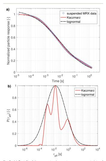
Fig. 3 (a) Best fit of the magnetorelaxometry measurement data of suspended nanoflowers using a lognormal distribution and using Kaczmarz' method. (b) The obtained relaxation time distributions corresponding to the fits in panel (a).
