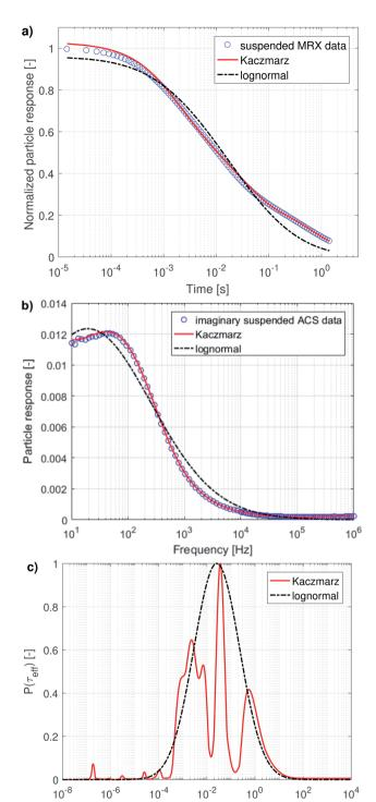
Fig. 5 Best combined fit to (a) the magnetorelaxometry measurement data and (b) imaginary part of the AC-susceptibility measurement data of suspended nanoflowers using a lognormal distribution and using Kaczmarz' method. (c) The obtained relaxation time distributions corresponding to the fits in panel (a and b)
