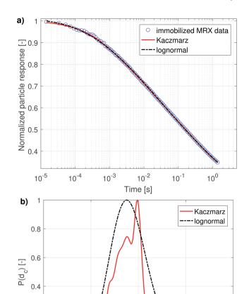
Fig. 2 (a) Best fit of the magnetorelaxometry measurement data of immobilised sample using a lognormal distribution and using Kaczmarz' method. (b) The obtained size distributions corresponding to the fits in panel (a).
