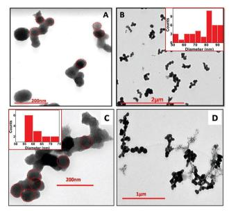
Fig. 5 TEM images of SnO<sub>2</sub> NPs at different magnification, synthesized via electron beam irradiation. (A) 35 kGy, (B) 72 kGy, (C) 107 kGy and (D) 143 kGy in the reline matrix.
