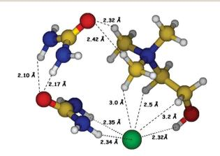
Fig. 1 Hydrogen bonded molecular structure of the deep eutectic
