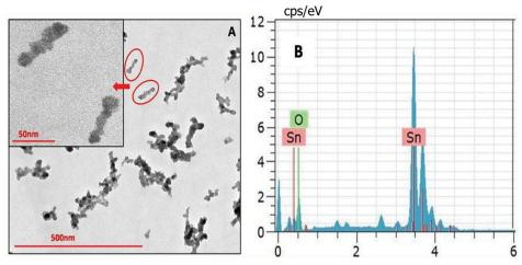
Fig. 6 (A) TEM image of SnO<sub>2</sub> NPs obtained via a solvothermal route in the reline matrix. (B) The EDX spectrum of the SnO<sub>2</sub> nanoparticles.
