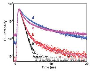
Fig. 8 Time resolved PL decay curve ( $\lambda_{\rm exc}$  = 280 nm) of SnO<sub>2</sub> nanoparticles at different emission wavelengths (a) IRF; (b) 320 nm; (c) 467 nm; and (d) 400 nm.
