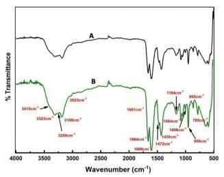
Fig. 9 FTIR spectra of (A) only reline and (B) reline containing dissolved SnCl<sub>2</sub>·2H<sub>2</sub>O and heated at 80 °C.
