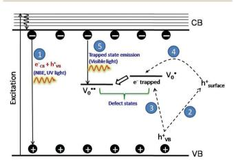
**Scheme 1** Schematic diagram depicting the possible pathways of emission in tin oxide nanoparticles.
