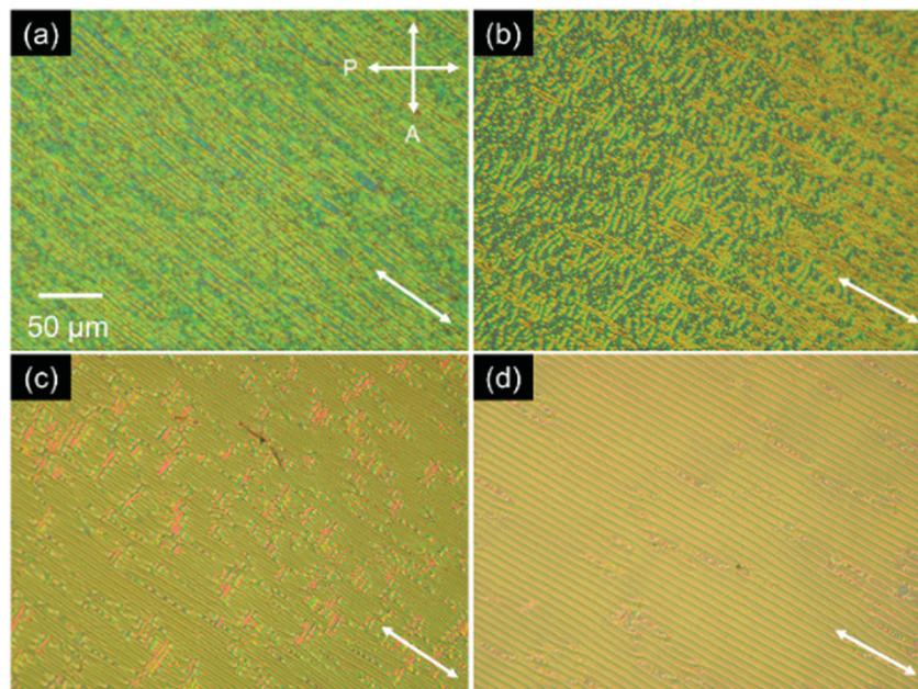
Fig. 4 POM images of the  $N_{TB}$  phases of (a) CBCOO4SCB, (b) CBCOO6SCB, (c) CBOCO4SCB, and (d) CBOCO6SCB in a uniaxially rubbed cell with planar alignment. The POM image in panel (a) is reproduced from ref. 53 with permission from Elsevier.
