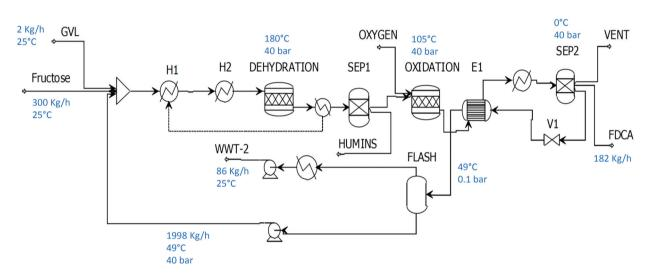
Fig. 5 The two stage water/GVL process for the synthesis of FDCA from fructose without product isolation.
