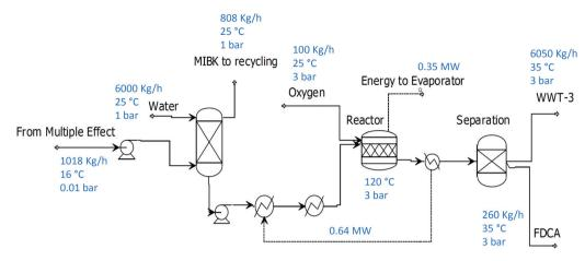
Fig. 4 Process flowsheet to produce FDCA by transfer of HMF to the water phase from MIBK, followed by oxidation.
