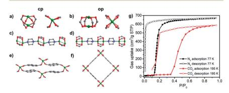
Fig. 10 Comparison of the closed (a, c, e) and open (b, d, f) phases of DUT-8(Ni); (g)  $N_2$  (77 K) and  $CO_2$  (195 K) sorption isotherms of DUT-8(Ni).
