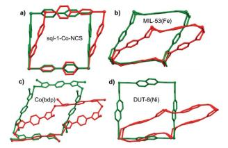
Fig. 21 Overlay comparison of closed (red) and open (green) phases of four switching CNs: (a) sql-1-Co-NCS; (b) MIL-53(Fe); (c) Co(bdp) and (d) DUT-8(Ni).
