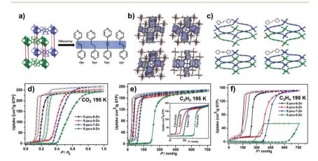
Fig. 11 (a) The two-fold interpenetrated structures of X-pcu-n-Zn; (b) as-synthesised "open" phases, X-pcu-n-Zn- $\alpha$ ; (c) activated "closed" phases, X-pcu-n-Zn- $\beta$ ; (d-f) CO<sub>2</sub>,  $C_2H_2$  and  $C_2H_4$  sorption isotherms on X-pcu-n-Zn- $\beta$  at 195 K. Reproduced from ref. 147 with permission; copyright: 2019, John Wiley & Sons, Inc.
