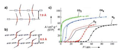
Fig. 18 Crystal structures of (a) open and (b) closed phases of [Cu(dhbc)<sub>2</sub>(bpy)] and (c) high pressure gas sorption isotherms of its activated phase at 298 K. Figure (c) is reproduced from ref. 65 with permission; copyright: 2003, John Wiley & Sons, Inc.
