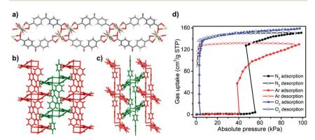
Fig. 19 (a) 1D double chain structure of [Cd(bpndc)]; (b and c) 2D bilayer structure of assynthesised and activated forms of [Cd(bpndc)(bpy)]; (d)  $O_2$ ,  $N_2$  and Ar sorption isotherms recorded on activated [Cd(bpndc)(bpy)] at 90 K.
