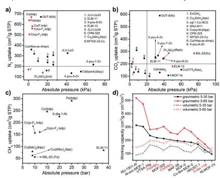
Fig. 22 Comparison of switching CNs with respect to (a) N<sub>2</sub> (77 K), (b) CO<sub>2</sub> (195 K) and (c) CH<sub>4</sub> (298/303 K) sorption. Black and red symbols denote CNs with type F-IV<sup>s</sup> and F-IV<sup>m</sup> isotherms respectively. For type F-IV<sup>m</sup> isotherms, only the switching pressures of the last step are shown. (d) Comparison of gravimetric and volumetric working capacities for CH<sub>4</sub> at 298 K between current benchmarks for switching and rigid CNs.
