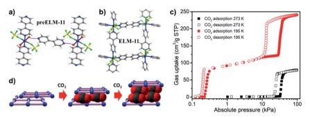
Fig. 16 The structures of (a) preELM-11 and (b) ELM-11; (c)  $\rm CO_2$  sorption isotherms of ELM-11 at 195 and 273 K; and (d) illustration of expansion/shrinkage of the adjacent layers in ELM-11. Figure (d) is reproduced from ref. 86 with permission; copyright: 2016, American Chemical Society.
