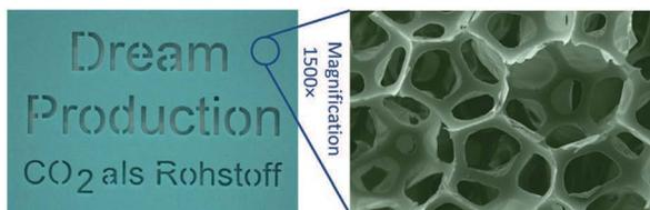
Fig. 7 Polyurethane foam made from polycarbonates that were synthesized with  $\text{CO}_2$ .<sup>104</sup> (Reproduced with permission by the publisher).
