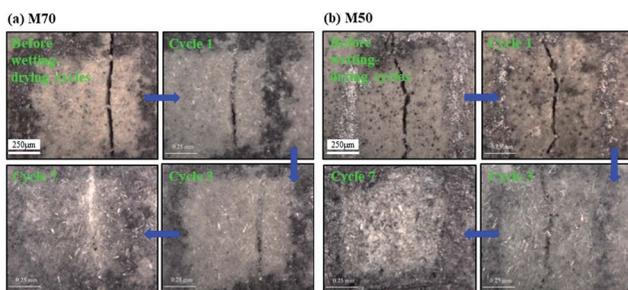
Fig. 5 Self-healing properties of highly ductile carbonated Engineered Cementitious Composite (ECC)<sup>52</sup> (reproduced with permission by the publisher).
