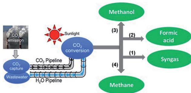
Fig. 6 Schematic illustration of a solar refinery system for converting CO<sub>2</sub> and wastewater into chemicals and fuels<sup>72</sup> (reproduced with permission from Energy in Frontiers).
